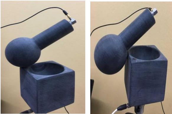
(c) Case 2: Femoral head outside the acetabulum (d) Case 3: Femoral head completely outside the acetabulum.
