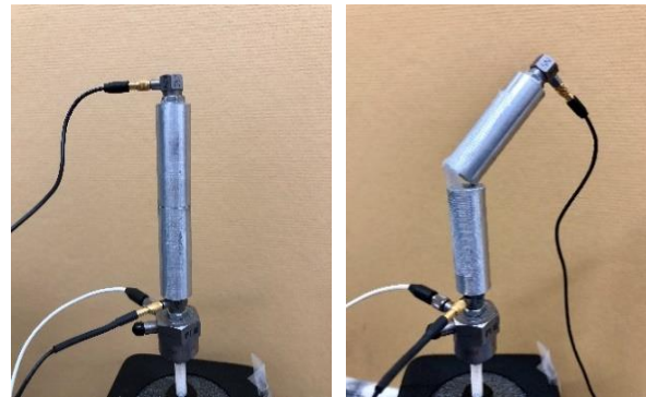
(a) Aluminum bars with 0 degree angle (b) Aluminum bars with 35 degree angle
