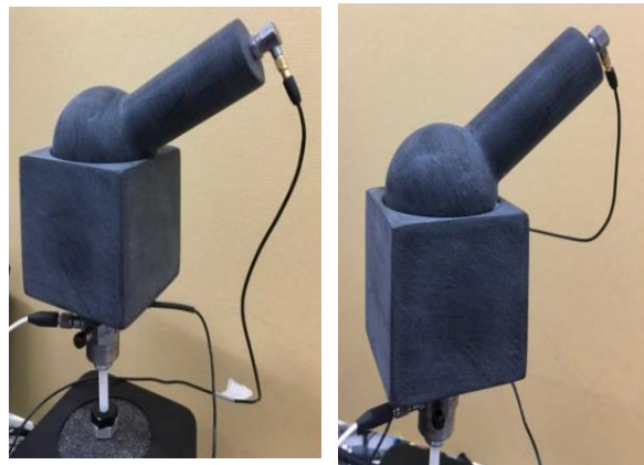
(a) Case 0: Femoral head completely inside acetabulum (b) Case 1: Femoral head partially inside acetabulum
