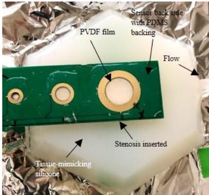
Figure 6. Banded silicone tubing embedded in silicone rubber was used as a vascular access phantom. Water was pumped through the phantom at physiologic flow rates and PAGs were recorded using each type of sensor.
