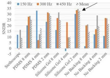
Figure 5. Sensors with 2 mm diaphragms had the highest SNDR and performed well at all three test frequencies.
