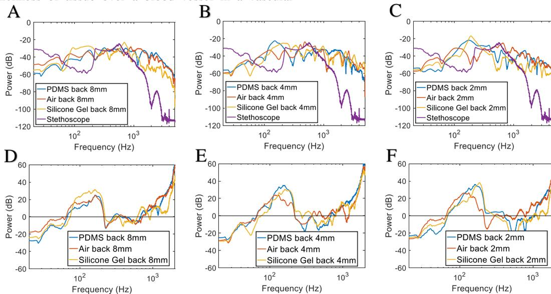
Figure 4. Frequency response comparison between sensors with different backing layers (A-C). When plotted relative to the stethoscope response, PVDF sensors showed enhanced mid-band and high frequency gain (D-F).
