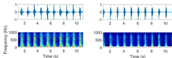
Figure 9. Time and wavelet scale representations of PAG recorded from (A) conventional stethoscope, and (B) the 2 mm sensor with silicone gel, both using FDLP systole pulse enhancement.
