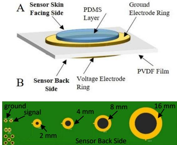
Figure 2. (A) Schematic structure of a sensor showing the PVDF film sandwiched between two electrodes and a layer of PDMS on the skin-facing side. (B) Layout of a sensor test board containing 2, 4, 8 and 16-mm diaphragm sizes.
