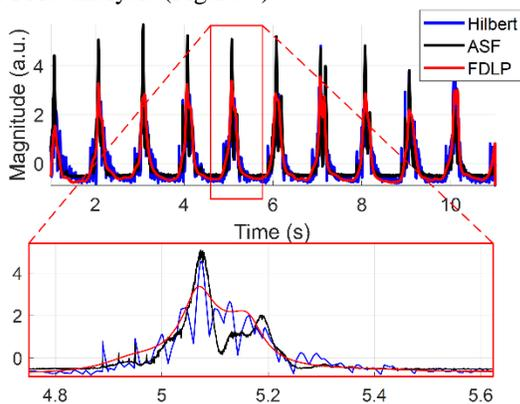
Figure 8. Analytical signals obtained from PAGs can include Hilbert envelope, auditory spectral flux, and FDLP-modeled envelopes. Of these signals, FDLP produced the smoothest response, permitting efficient feature extraction.
