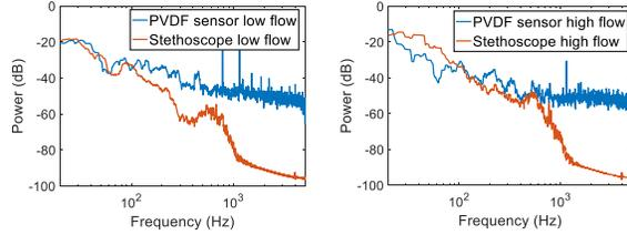
Figure 7. The frequency spectra of PAGs recorded using i) the 2 mm sensor with silicone and polyimide tape backing, and ii) the stethoscope, at (a) low, and (b) high flow rates.
