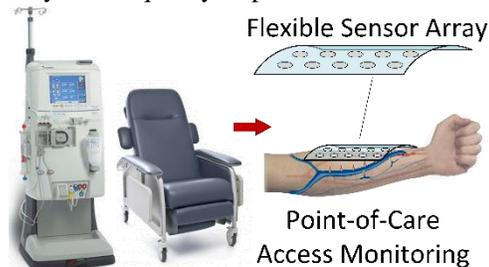
Figure 1. Dialysis vascular access monitoring with a flexible array of sensors capable of recording and processing blood flow sounds to determine stenosis risk.
