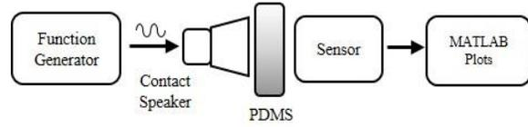
Figure 3. Test setup for frequency response measurements.
