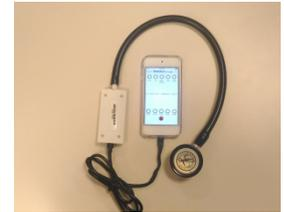
Figure 1. The stethoscope accessory with the recording application.
